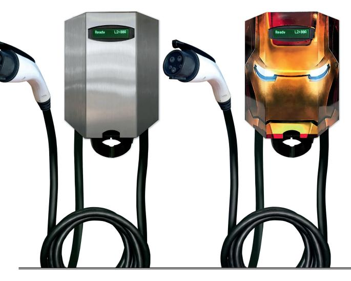
custom-made enclosure with an inner polycarbonate layer surrounded by aluminum. It's built to be durable, with a standard T6061 black anodized aluminum can that adheres to National Electrical Manufacturers Association (NEMA) Type 4X standards. WattZilla says you can drive over it with a truck, and it's designed to withstand a two-thousand-pound test. On the other end is a J1772 coupler.
